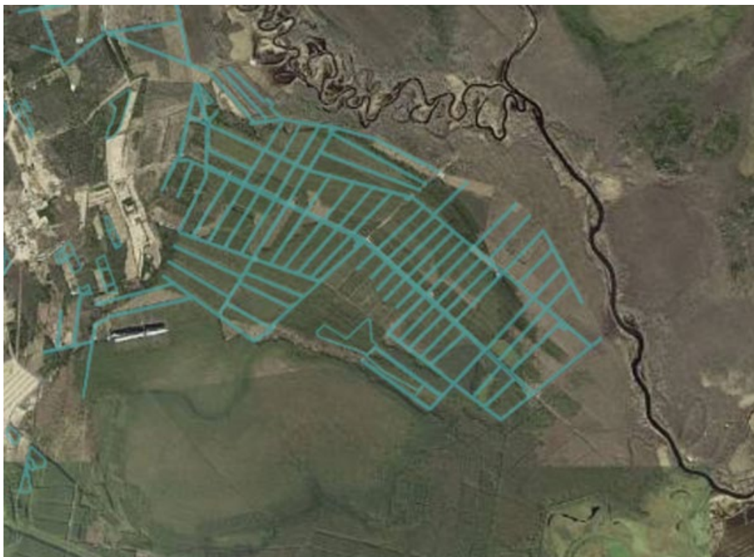
Photo 34: Satellite image of the state forest in Meleski with the ditches planned for renovation in light blue.
